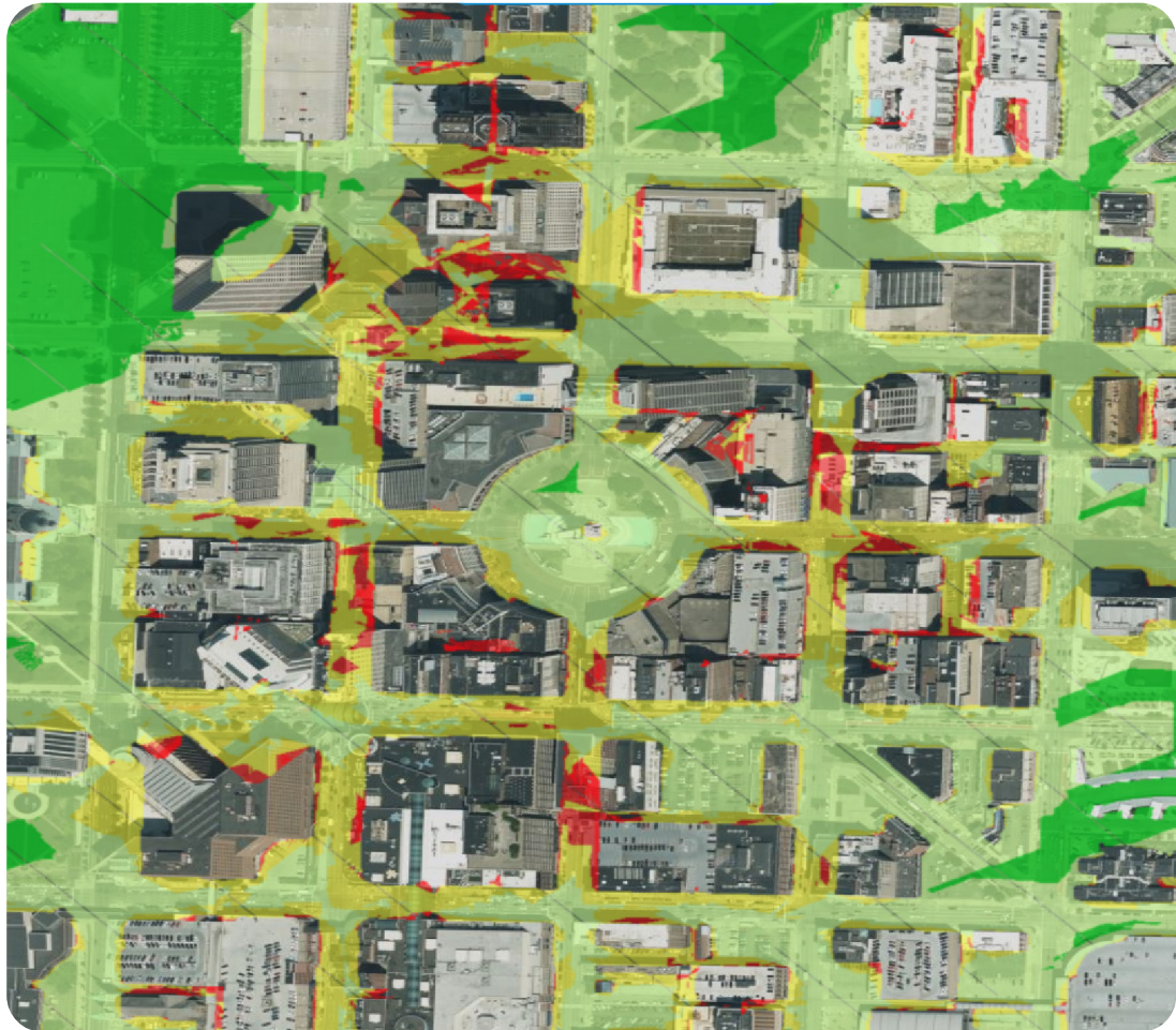
Figure 3: Signal coverage in downtown Indianapolis for a multi-GNSS receiver
